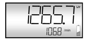
**Accumulative Total** The 8 digit display can be programmed for up to 3 decimal places. Reset is only possible when in the program mode which can be PIN protected for security.
