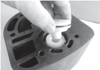
Step 3b From the opposite side we remove both cap and air valve shaft
