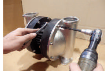
Step 3 Untie one of the two housings, by untying the screws gradually and cyclically.
