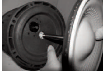
Step 5 Untie the opposite housing and pull the diaphragm along with the shaft outwards. Remove the diaphragm from the shaft
