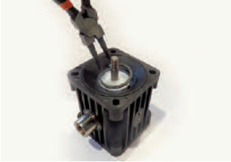
Step 1 Insert the air control unit in the central block. Mount the retaining ring to the central block
