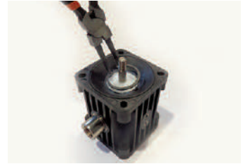
Step 6 Disassemble the retaining ring of the air control unit .
