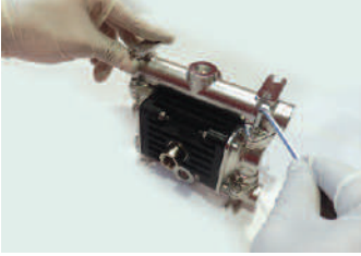
Step 1 Disassemble the discharge manifold by untying the retaining screws
