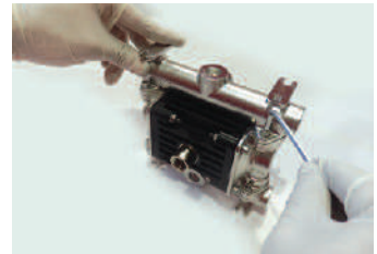
Step 6 Install the suction manifold onto the pump and the tighten the screws. Follow the same procedure to install the discharge manifold
