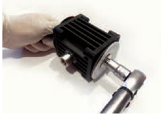
Step 2 Install the outer pistons, diaphragms and screw the external caps
