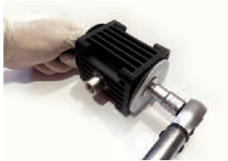
Step 5 Disassemble the diaphragms by untying the external caps that retain the diaphragms and remove the diaphragms and the outer pistons
