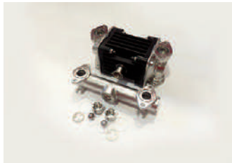
Step 5 Install into the pump housings the balls , seats and orings
