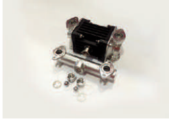
Step 2 Remove the discharge manifold , the seats , the balls and the o-rings of the valves. Follow the same procedure (steps 1 & 2) to remove the suction manifold as well.
