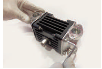
Step 3 Disassemble the pump housing by untying the retaining screws
