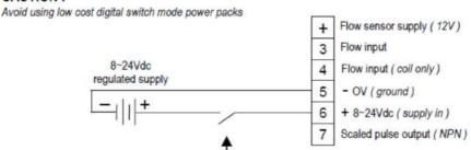
Note: Powering the instrument from an external DC source will cause the backlighting feature to turn on, if this is not desirable at all times then install a power isolation switch in series with the DC power source as shown.
