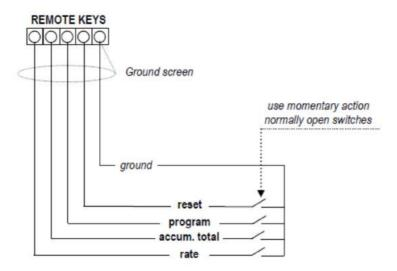
Wiring requirements: Use multi-core screened twisted pair instrument cable (0.25-0.5mm2) for electrical connection between the instrument and any remote flow meter or receiving instrument. The screen needs to be earthed to the signal ground of the receiving instrument only to protect the transmitted signal from mutual inductive interference.
